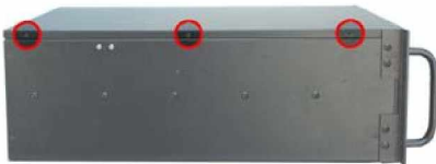
Figure 2: Top Cover Retention Screws
