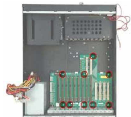
Figure 13: Backplane Retention Screws
