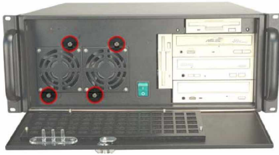
Figure 31: Fan Bracket Thumbscrews
