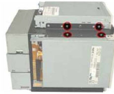
Figure 26: FDD Retention Screws
