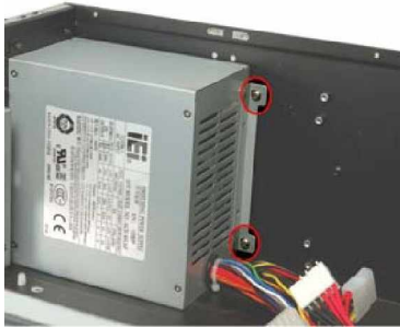
Figure 6: PSU Internal Retention Screws
