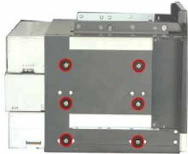
Figure 23: 5.25" Optical Drive Retention Screws
