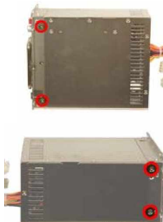
Figure 8: Redundant PSU Clamp Retention Screws
