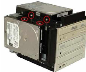
Figure 27: HDD Retention Screws
