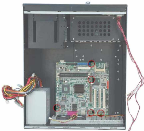
Figure 43: Motherboard Retention Screws
