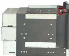
Figure 24: Top 3.5" Drive Bay Front Cover Retention Screws
