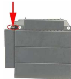
Figure 21: Left 3.5" Drive Bay Front Cover Retention Screws
