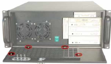
Figure 33: Fan Filter Bracket Retention Screws
