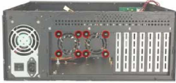
Figure 36: Fan Retention Screws
