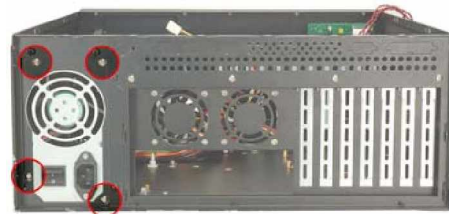
Figure 5: PSU Retention Screws at the Rear
