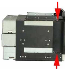
Figure 25: Left 3.5" Drive Bay Front Cover Retention Screws
