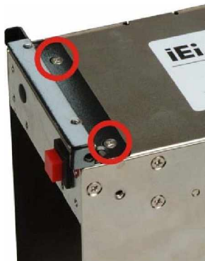
Figure 9: Attach the PSU Bracket to the PSU
