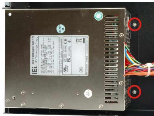
Figure 12: Secure the PSU Rear Bracket
