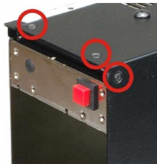
Figure 11: Mount the PSU in the Chassis
