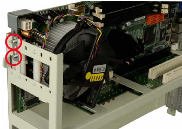
Figure 20: Insert Two Shock Absorber Retention Screws
