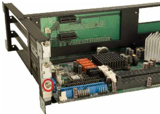
Figure 19: Secure the CPU Card to the Backplane Bracket
