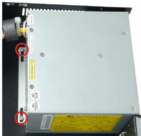
Figure 7: Insert PSU Rear Bracket Screws and Nuts
