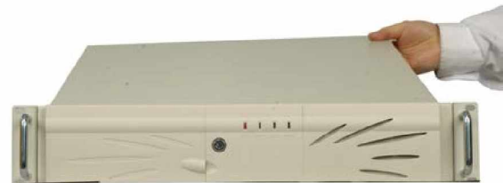
Figure 5: Remove the Top Cover
