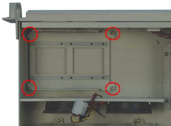
Figure 23: 3.5" HDD Bracket Retention Screws
