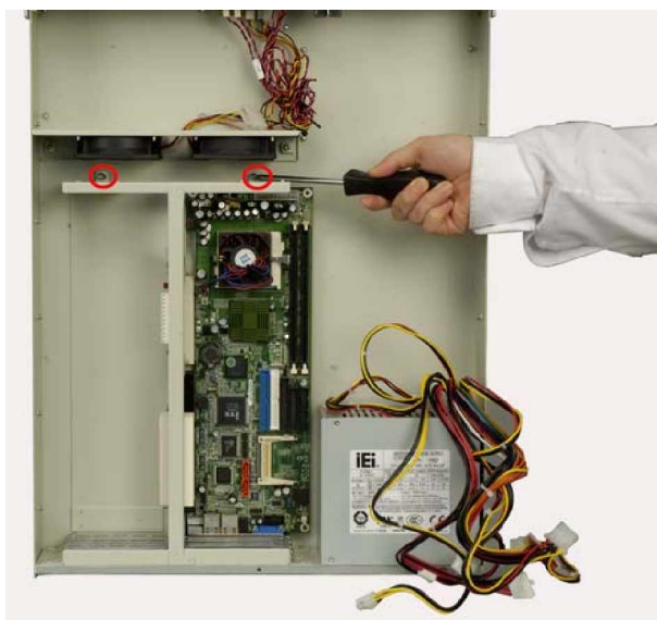
Figure 21: Backplane Bracket Chassis Retention Screws
