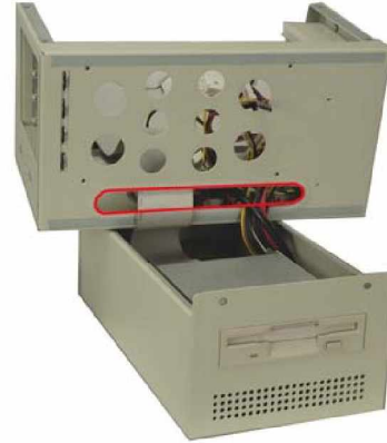
Figure 14: Run the Cables through the Elliptical Hole
