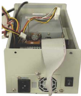
Figure 13: HDD Power Cable and IDE/SATA Connector
