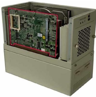
Figure 21: Slide the CPU Card into the Socket
