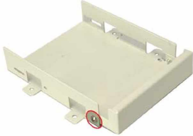
Figure 11: 3.5" FDD Bracket Front Cover Retention Screw
