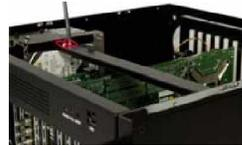
Figure 5: Remove the 2 Hold-Down Clamp Retention Screws
