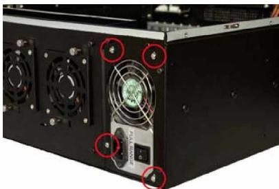
**Figure 8: Insert PSU Retention Screws**
