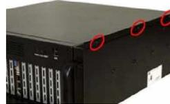
Figure 3: Top Cover Retention Screws
