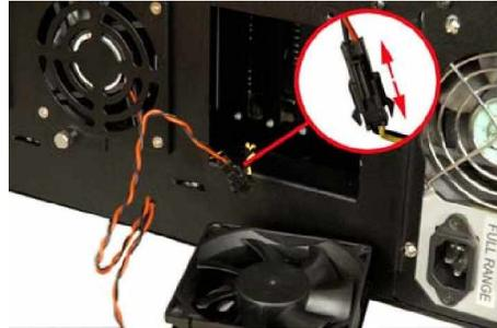
Figure 23: Unplug the Fan Power Cable
