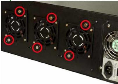
Figure 22: Locations of the Fan Bracket Thumbscrews
