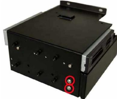
Figure 17: Remove the 4 Retention Screws on the Sides of the Main Bracket
