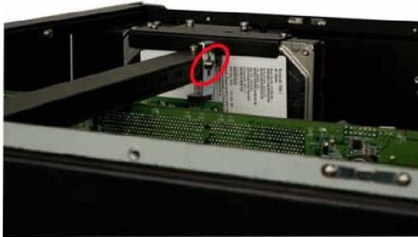
Figure 21: PCI/ISA Card Shock Absorber
