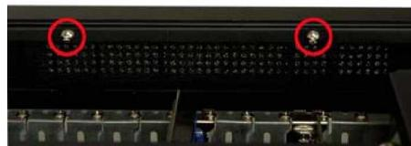
Figure 25: Remove the Fan Filter
