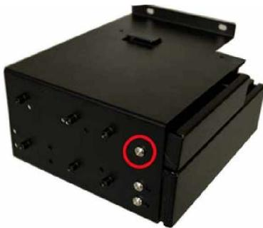
Figure 15: Remove the Front Metal Cover Retention Screws
