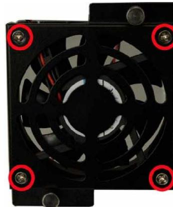
Figure 24: Remove the Fan Retention Screws
