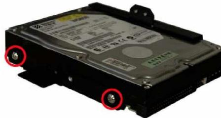
Figure 13: Insert 4 HDD Retention Screws
