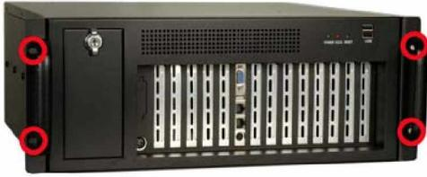
Figure 26: Locations of the 4 Mounting Holes
