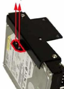
Figure 20: Hold-Down Clamp Retention Screw Holes in the Clip of the Side HDD bracket
