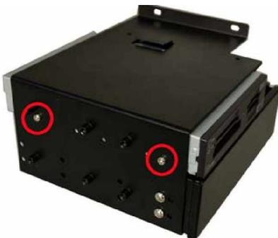
Figure 16: Insert Four 3.5" Drive Retention Screws
