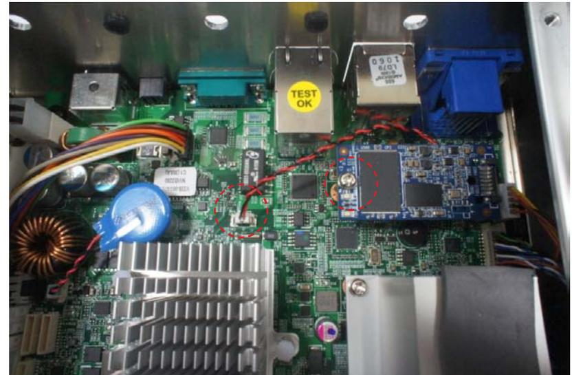
3. Tighten the screw back on the top of the copper post.
