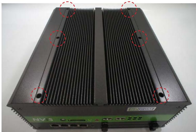
2. Lift up the cover and remove it from the chassis.
