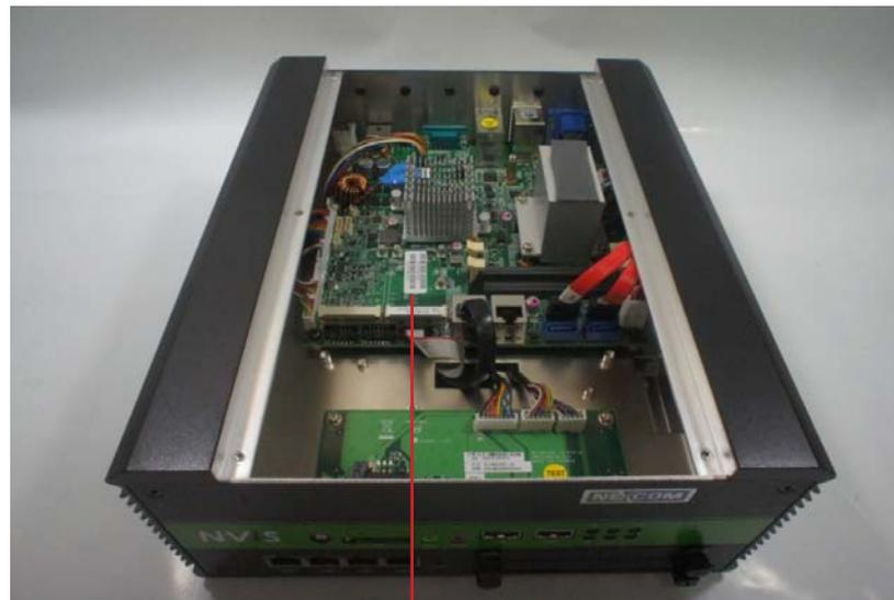
Mini-PCI Slot for WLAN
