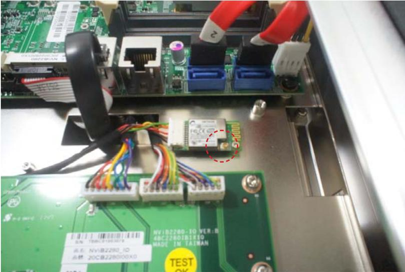
3. Tighten a screw on the mounting hole to secure the module.
