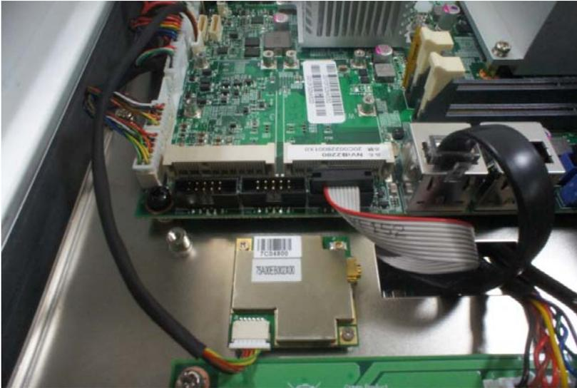
3. Tighten screws on the mounting holes to secure the module, and connect the GPS module connector to the J8 (GPS connector) connector on the motherboard.
