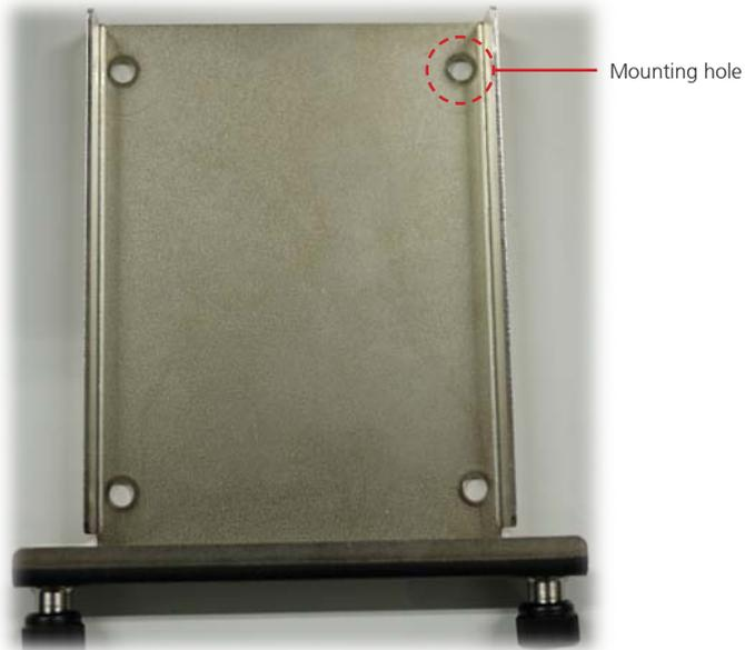
4. Tighten the hard drive with 4 screws, make sure the SATA connector is facing towards the end of the drive bay.
