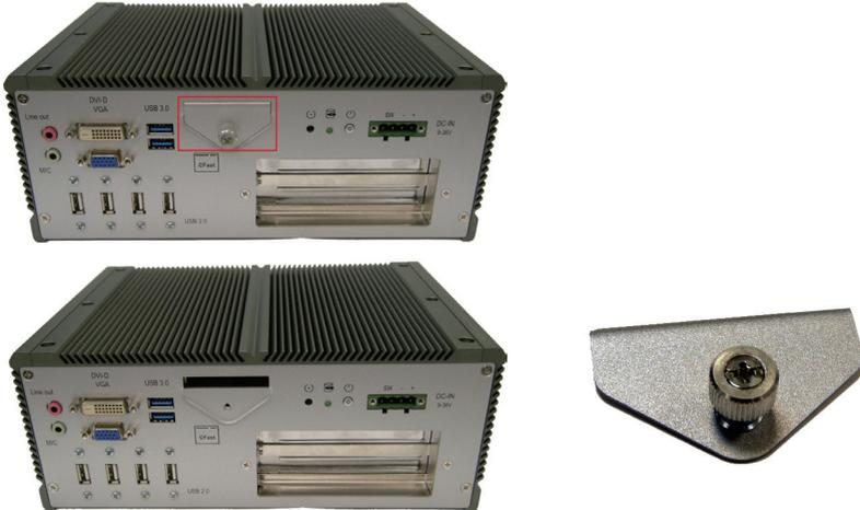
2. Insert your CFast card into the slot according to the illustration by the card holder. Push it inward until you hear a click. Close the card door and screw it on clockwise.
