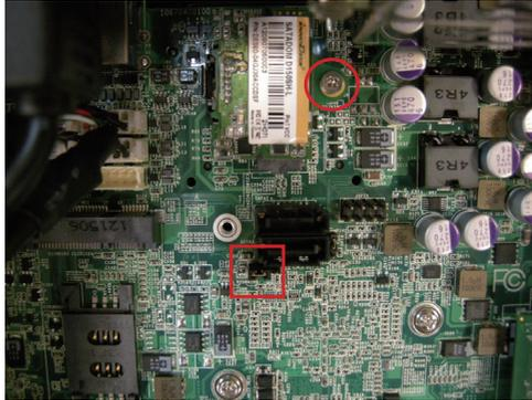
4. Reinstall bottom cover back to its original place. Be careful not to press SATA cable in the process and not to pull it away next time you remove bottom cover.
