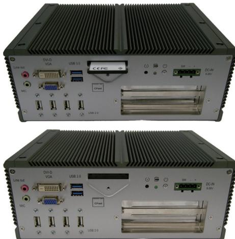
3. To remove the CFast/SIM card, follow step 1 and 2 above. And then push card inward to pop-out it from the slot.
