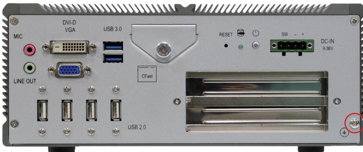
1. As the figure illustrates above, remove the ground screw located on the bottom-right of the rear panel.
