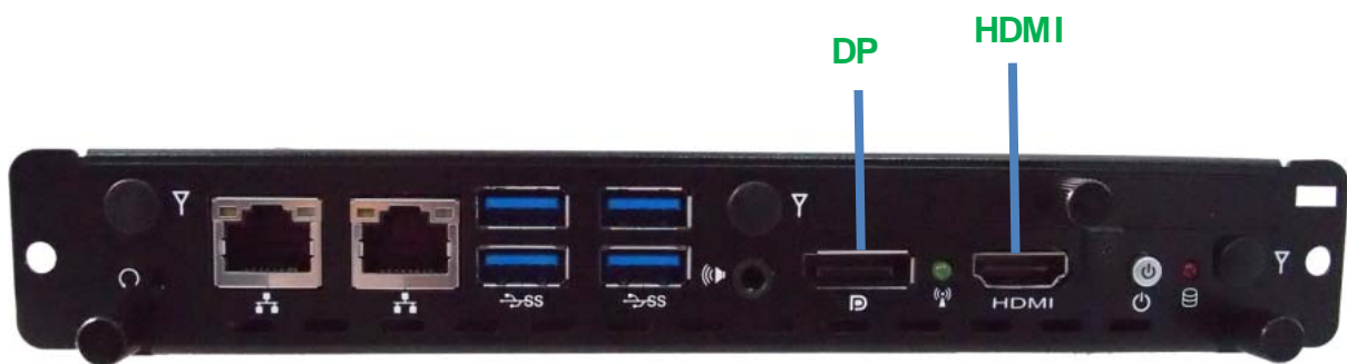
Figure 3 Connect the DP/ HDMI cable
