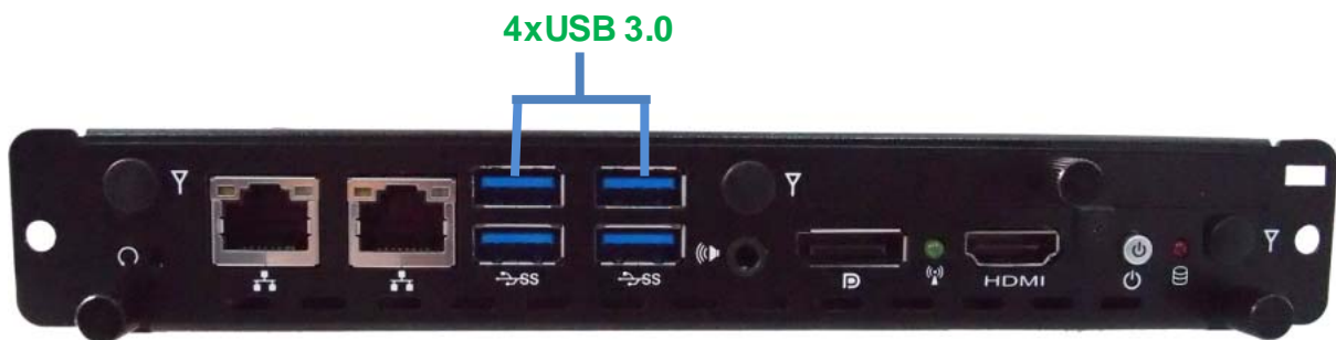
Figure 4 Connecting USB mouse & keyboard
