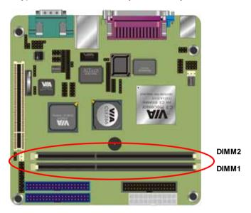
The motherboard support DDR200/266 SDRAM. If you install higher frequency RAM module more than 266MHz, the system will force it to run under 266MHz.
