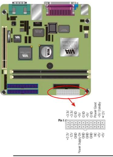
Incorrect installation of the power supply could result in Warning: serious damage to the motherboard and connected peripherals. Make sure the power supply is unplugged from the AC outlet before connecting the leads from the power supply.
