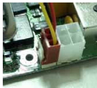
4. Connect the fan connector on CPUFAN
