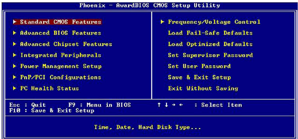
Figure 4-1 CMOS Setup Utility Main Screen
