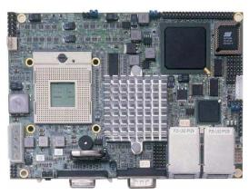
The 2807640 is an Intel® 852GME GMCH and 2807650 is an Intel® 852GM GMCH chipset-based board designed. The 2807640/2807650 is ideal all-in-one embedded engine board. Additional features include an enhanced I/O with CF, CRT/LVDS, dual LAN, audio, 4 COM, and USB2.0 interfaces.
