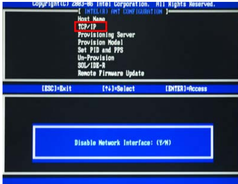
Figure 6-9: Enable Network Interface
