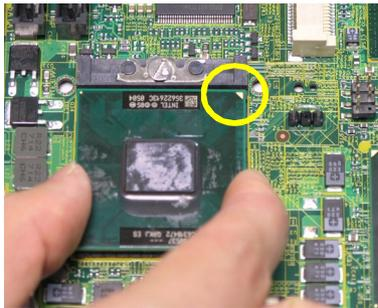
4. On the front end of the CPU socket is a locking mechanism designed into the form of a screw head. Make sure that you actuate or deactivate this mechanism with a screwdriver before and after installing the CPU.
