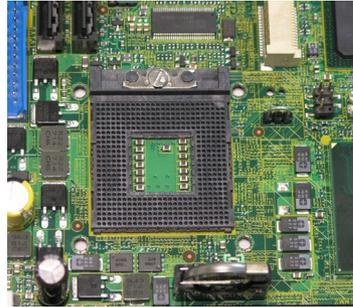
2. Place the CPU on top of the socket. Make sure that you align the gold arrow on the CPU with the arrow key on the socket.
