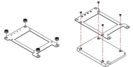
2. Follow the photo instruction install the HDD\_KIT onto the chassis.
