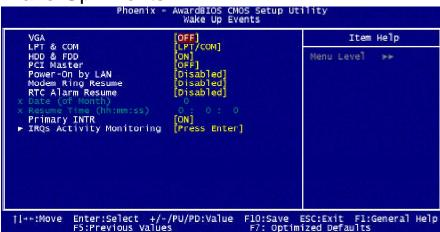
**VGA** --->When ON, an event occurring on each listed device restarts the global timer for Standby mode.
