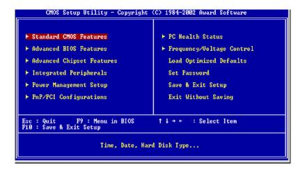
Once you enter the AwardBIOS<sup>TM</sup> CMOS Setup Utility, the Main Menu will appear on the screen. The Main Menu allows you to select from several setup functions and two exit choices. Use the arrow keys to select among the items and press <Enter> to accept and enter the sub-menu.
