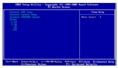
Current CPU Temperature Show you the current CPU temperature
