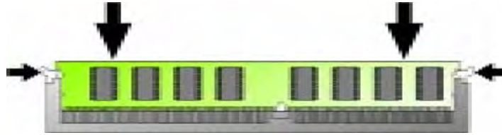
Figure 3-3 : How to Install DIMM (3)
