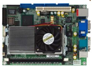
The 3301500 is an Intel<sup>®</sup> 82855GME/ICH4 chipset-based board designed for PCI Bus PGA 479 Intel<sup>®</sup> Pentium<sup>®</sup> M 1.2~1.7GHz CPU compatibility. These features combine and make the 3301500 an ideal all-in-one industrial single board computer. Additional features include and enhanced I/O with CRT/LVDS Panel, Giga LAN, audio and USB2.0 ports interface.
