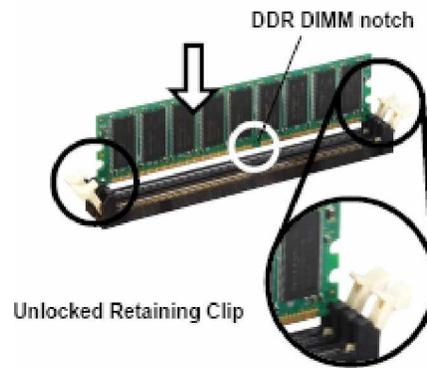
Slowly slide the DIMM module along the plastic guides on both ends of the socket, then press the DIMM module right down into the socket, until you hear a 'click' sound. This is when the two handles have automatically locked the memory module into the correct position of the DIMM socket. To remove the memory module, just push both handles outward, and the memory module will be ejected by the mechanism in the socket.
