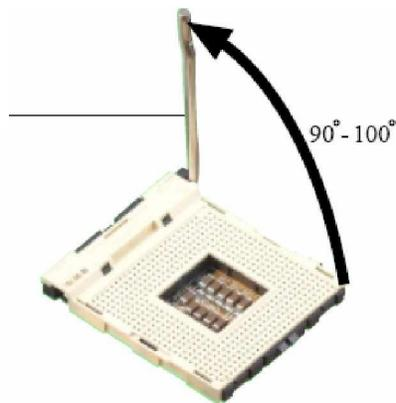
Step 2: Align the corner having the triangle marking on the processor with the corner where the lever is attached to the socket
