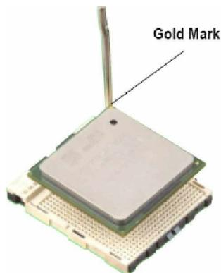
Step 3: Lower the lever to its original position
