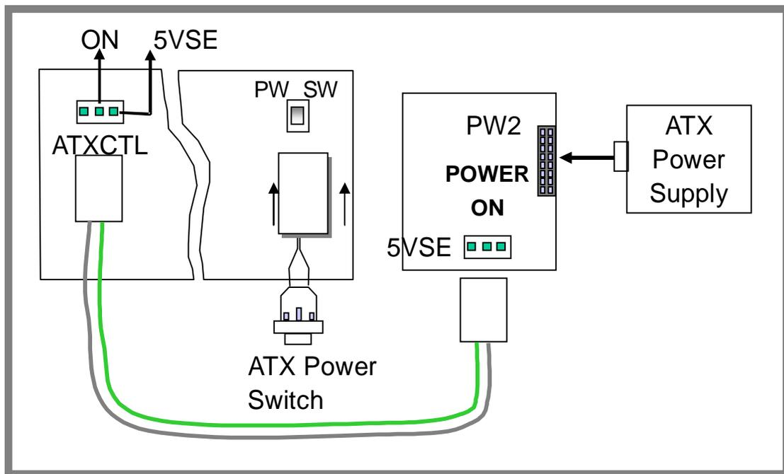
Step 2. Connect the ATX power button switch to the PW\_SW (power button). And connect the power cable from Backplane to ATXCTL connector of CPU card.
