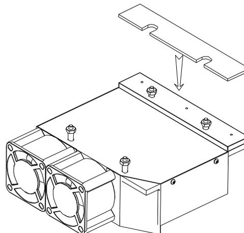
6) Place the cooler backplate on the backside of the 3301611.
