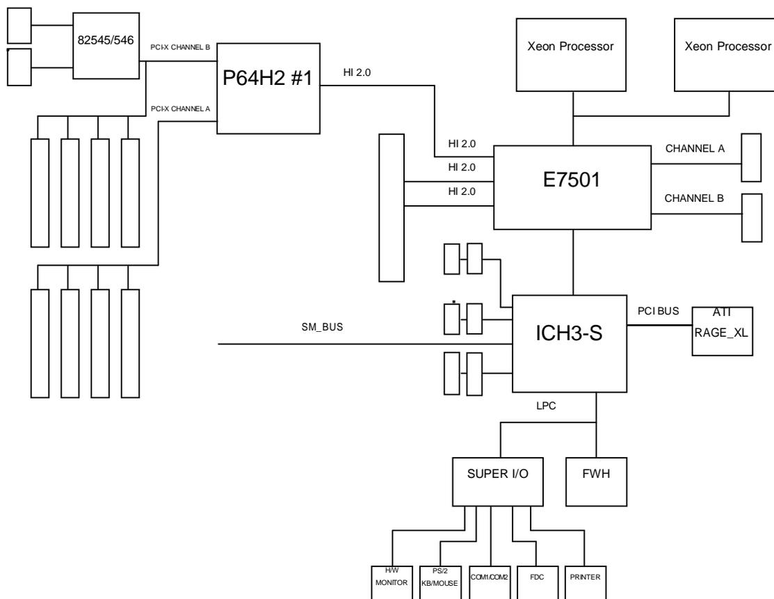
Figure 1-1 System Block Diagram of 3301611
