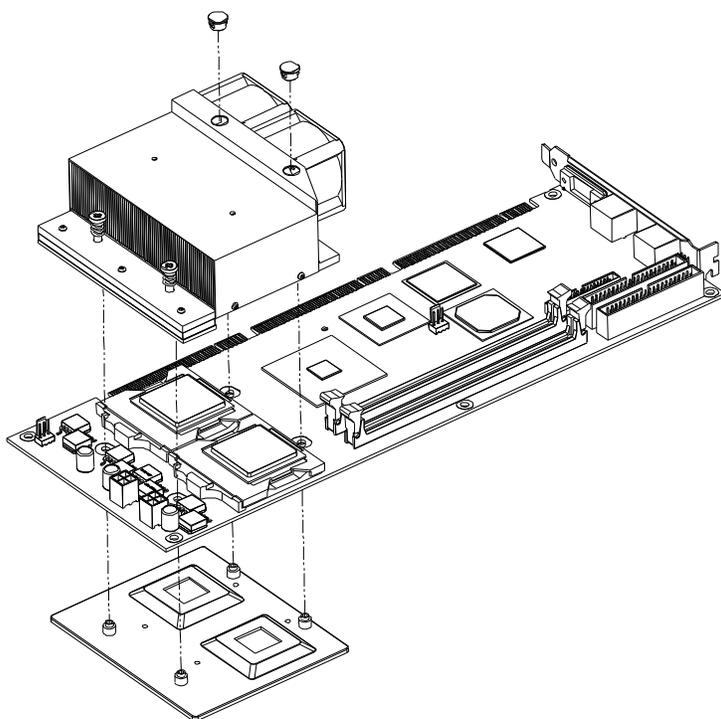
8) Install the CPU cooler on the SBC (Cooling fans nearest the DIMM sockets).
