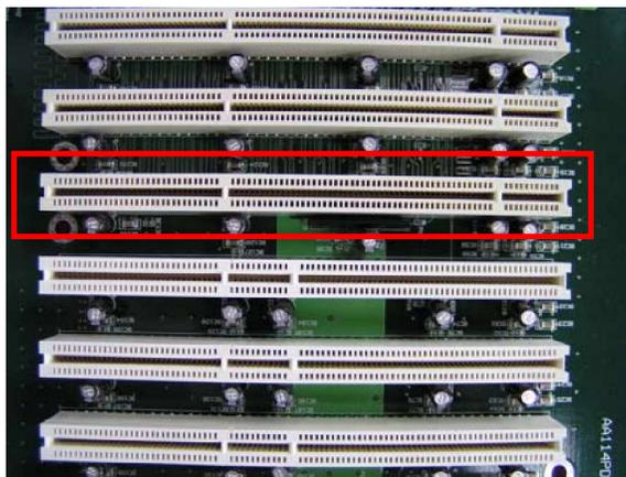
The 5V, 64 bit PCI Slot
