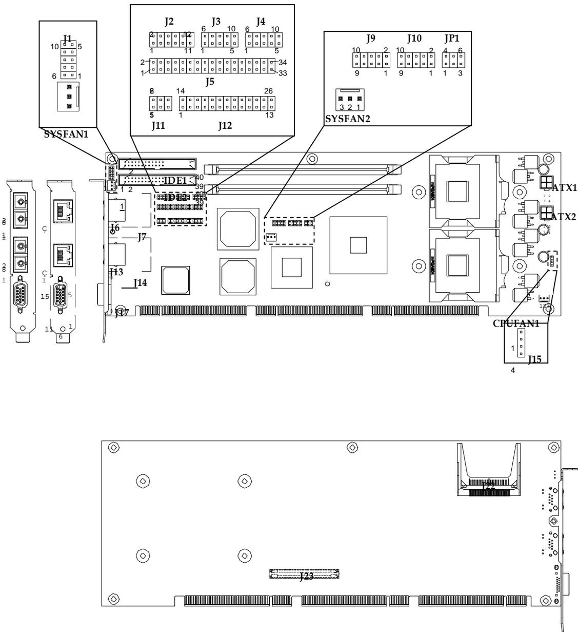
Figure 2-1 Jumper/Connector Locations for the 3301611
