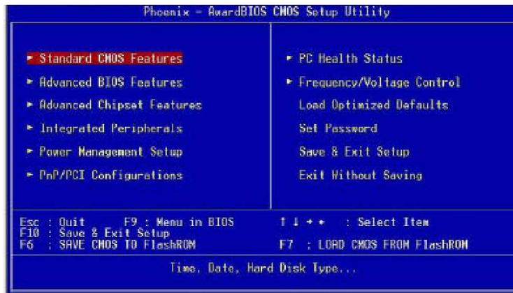
Once you enter the AwardBIOS<sup>®</sup> CMOS Setup Utility, the Main Menu will appear on the screen. The Main Menu allows you to select from several setup functions and two exit choices. Use the arrow keys to select among the items and press <Enter> to accept and enter the sub-menu.
