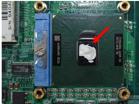
Figure 3-9: How to Install CPU (3)
