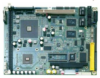
The 3302120 is a VIA CX700 chipset-based board designed. The 3302120 is an ideal all-in-one embedded engine board. Additional features include an enhanced I/O with CF, CRT/LVDS, TV-Out, dual GB LAN, audio, SATA, 4 COM, USB2.0, and PC/104 interfaces.
