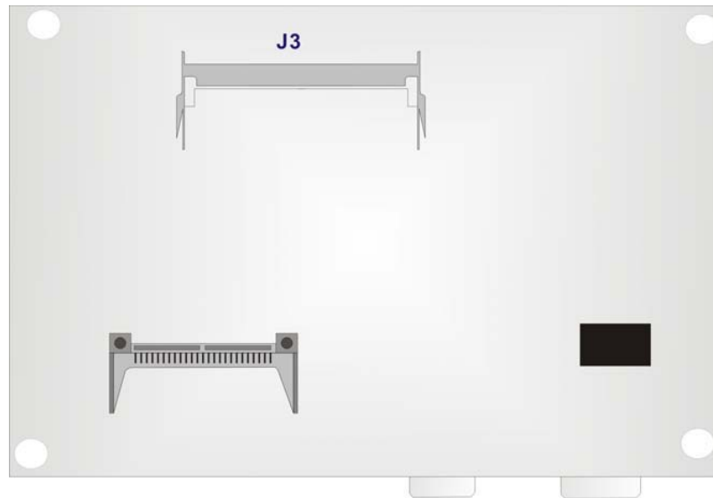
Figure 3-10: SODIMM Socket Location (Solder Side)
