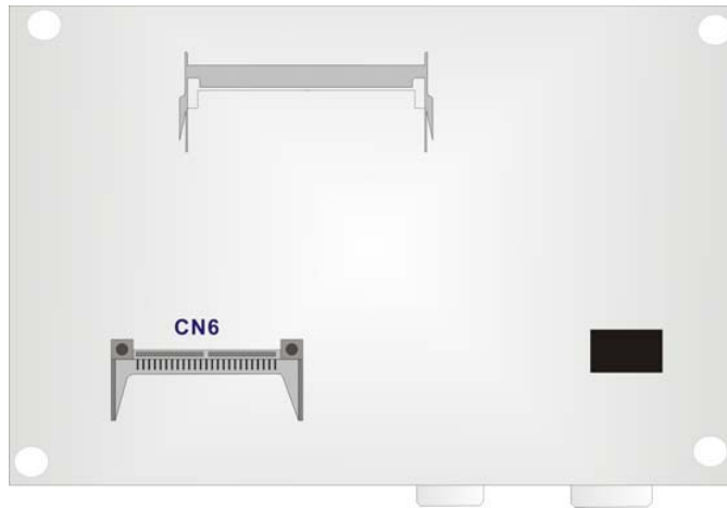
Figure 3-9: CFII Socket Location (Solder Side)
