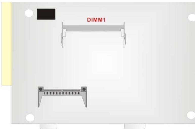
**Figure 3-7: SODIMM Socket Location (Solder Side)**
