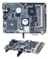
The 3304120 is a 100MHz FSB VIA CLE266/VT8235 chipset-based board designed for ULV Intel® Celeron® processor 400/650MHz. These features combine and make the 3304120 an ideal all-in-one industrial single board computer. Additional features include an enhanced I/O with CompactFlash reader, PCMCIA, CRT/Panel, audio, LAN, TV-Out, 4 COM, and USB2.0 interfaces.
