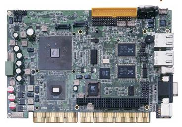
The 3301284/3304284 is a VIA CX700 chipset-based board designed. The 3301284/3304284 is an ideal all-in-one single board computer. Additional features include an enhanced I/O with CF, CRT/LVDS, dual LAN, audio, SATA, 4 COM, USB2.0, and PC/104 interfaces.
