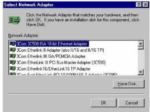
5. Setup now asks you for the location of the driver. When you have entered the new driver path, press on the OK button to continue.
