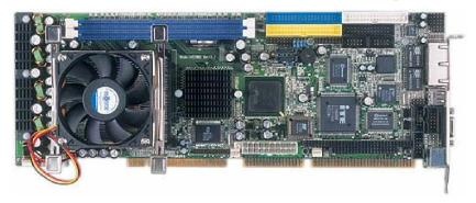
The 3307566 is an Intel® 82865GV/82801EB chipset-based board designed for PICMG Bus PGA 478 Intel® Pentium® 4 CPU with speed of up to 3.2GHz CPU. The combination of these features makes the 3307566 an ideal all-in-one industrial single board computer. Additional features include an enhanced I/O with CRT/LVDS Panel, TV-Out, dual Giga LAN, audio, serial ATA, 4 COM port interface, and more.
