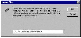
6. When Setup finds the information it needs about the new driver, it will display the device it found on the following screen. If using 82562EZ, please choose "Intel(R) PRO/100 Family Adapter". If using 82540EM or 82547EI, please choose "Intel(R) PRO/1000 Family Adapter". Press on the OK button to accept and proceed.
