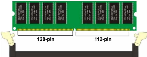
Please check the pin number to match the socket side well before installing memory module.
