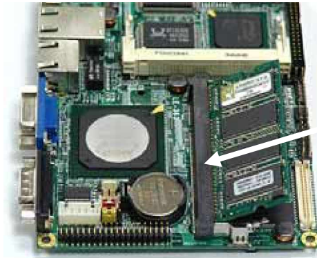
(1. Insert the DDR SO-DIMM module into the socket at 45 degree)
