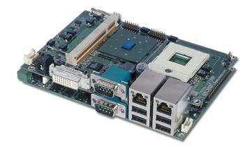
The 3307621 is an Intel<sup>®</sup> 82852GM/82801DB chipset-based board designed for PCI-ISA Bus PGA 479 Intel<sup>®</sup> Pentium<sup>®</sup> M 1.3~1.8GHz CPU/Mobile Celeron<sup>®</sup> M 600MHz low power embedded CPU compatibility. The combination of these features makes the 3307621 an ideal all-in-one industrial single board computer. Additional features include an enhanced I/O with CompactFlash, DVI-I/CRT/LVDS Panel, dual LAN, audio, 4 COM and USB2.0 port interface.
