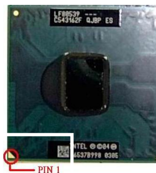
Figure 2. CPU's pin 1 mark
