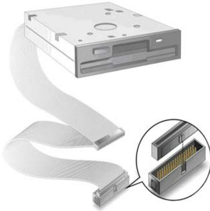
Figure 5-9: FDD Cable Connection
