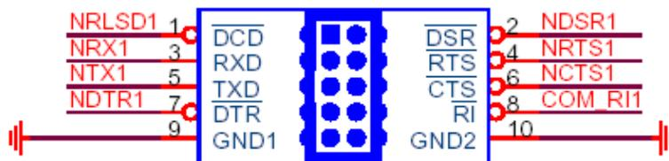
Figure 3-22: RS-232 Serial Port Connectors Location
