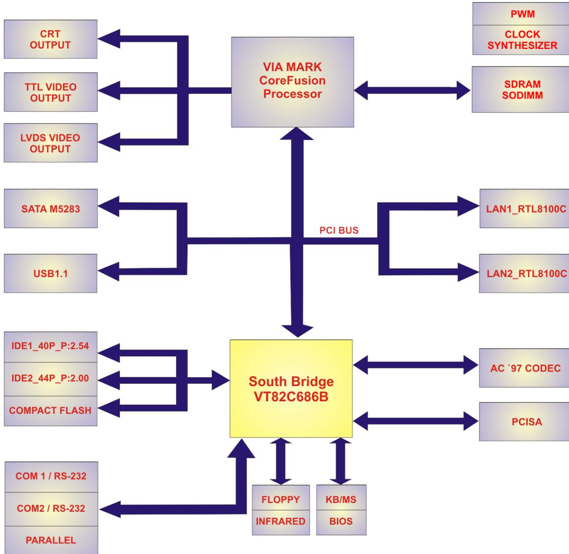
Figure 2-1: Data Flow Block Diagram
