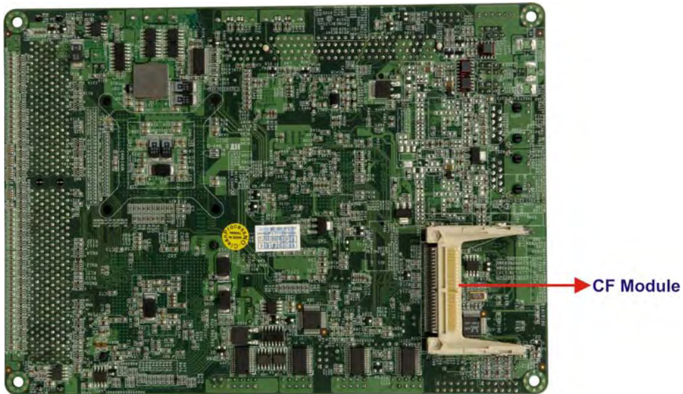
Figure 1-2: 3308040 Solder Side Overview
