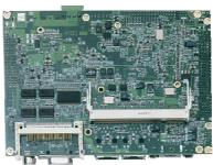
The 3308220 is a VIA CX700 chipset-based board designed. The 3308220 is an ideal all-in-one embedded engine board. Additional features include an enhanced I/O with CF, CRT/LVDS, TV-Out, dual LAN, audio, SATA, 4 COM, USB2.0, and PC/104 Plus interfaces.
