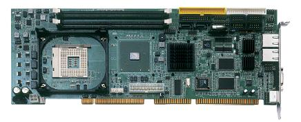
The 3308270 is an Intel® 915GV GMCH chipset-based board designed. The 3308270 is an ideal all-in-one PICMG Bus SBC. Additional features include an enhanced I/O with CF, CRT/LVDS, dual GB LAN, audio, SATA, COM, and USB2.0 interfaces.
