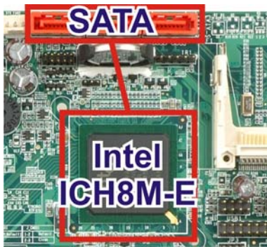
Figure 2-14: SATA Drive Connectors
