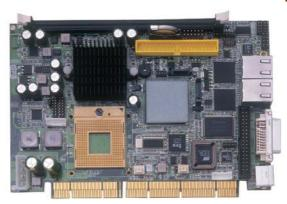
The 3308350 is an Intel® 945GME GMCH chipset-based board designed. The 3308350 is an ideal all-in-one PCI-ISA Bus single board computer. Additional features include an enhanced I/O with CF, DVI-I/CRT/LVDS, dual GB LAN, audio, SATA, COM, and USB2.0 interfaces.
