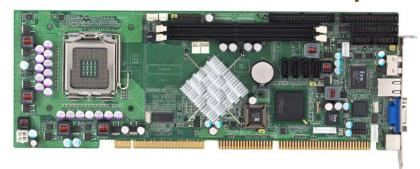
The 3312620 is an Intel® 915GV GMCH/ICH6 chipset-based and 3312620 is an Intel® 915GV GMCH/ICH6 chipset-based board designed PICMG Bus SBC. 3312620 provides Intel® Pentium® 4/Celeron® D processor 2.4~3.8GHz. The combination of these features makes the 3312620 an ideal all-in-one industrial single board computer. Additional features include an enhanced I/O with CRT, LAN, audio, SATA, 2 COM, IrDA and USB2.0 port interface.
