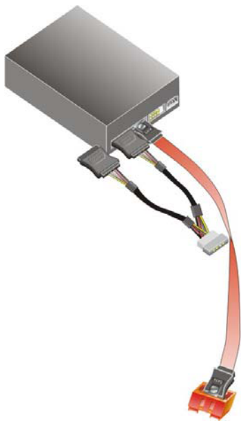
Figure 5-9: SATA Power Drive Connection
