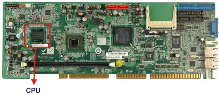
Figure 2-4: Intel® Atom™ N270 CPU
