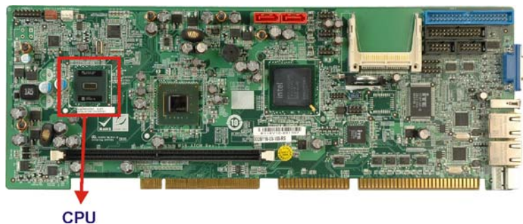
Figure 2-4: Intel® Atom™ N270 CPU
