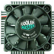
CPU Cooler x 1 (OHS-P-M-H)
